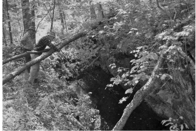
FIGURE 15. Bill Mueller of Colton and George Perrson of Star Lake (upper left corner) gaze into a water-filled shaft on the east side of Jayville hill, probably Hart No. 1 mine. The inclined shaft was said to follow a rich shoot of iron ore dipping down to the northwest (to the right) for 300 ft. Photo by J. Carl, May 20, 2009.
