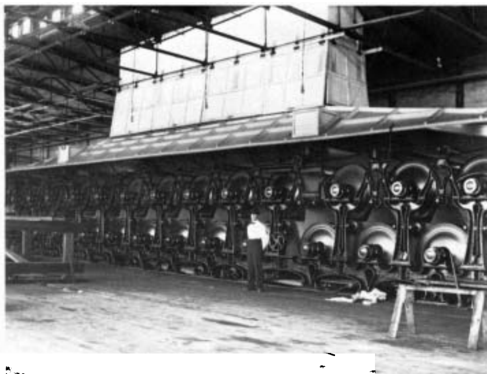
Interior view of the Pyrites mill showing the Fourdrinier machine. (Photograph courtesy of the Canton Municipal Museum)
