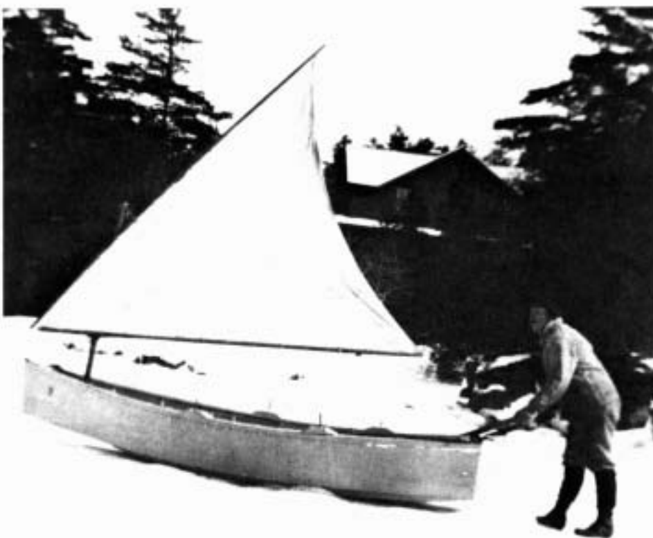
Getting supplies across the ice to Crossover Island: a small sled used about 1910 and a punt equipped by D. D. Hill with runners, sail, and handle. (Photographs courtesy of Ralph E. Hill)
