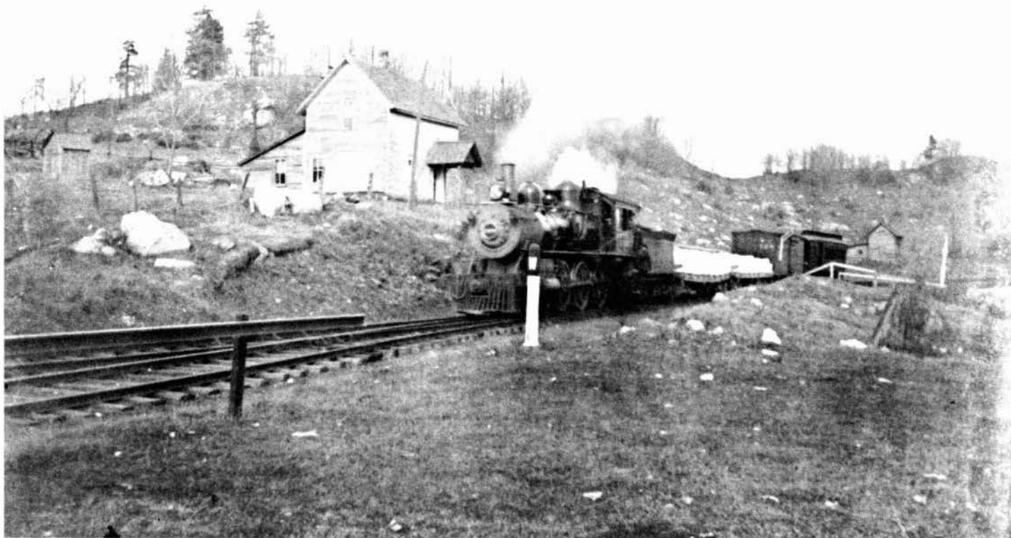
N.Y.C. & H.R. locomotive #2029 with combination train #995 [passenger and freight] near Talcville westbound to Gouverneur from Edwards. Talc ore on flat cars destined to Hailesboro mills, early 1900. Passenger-baggage-express-mail car on rear. (Photo courtesy of author).
